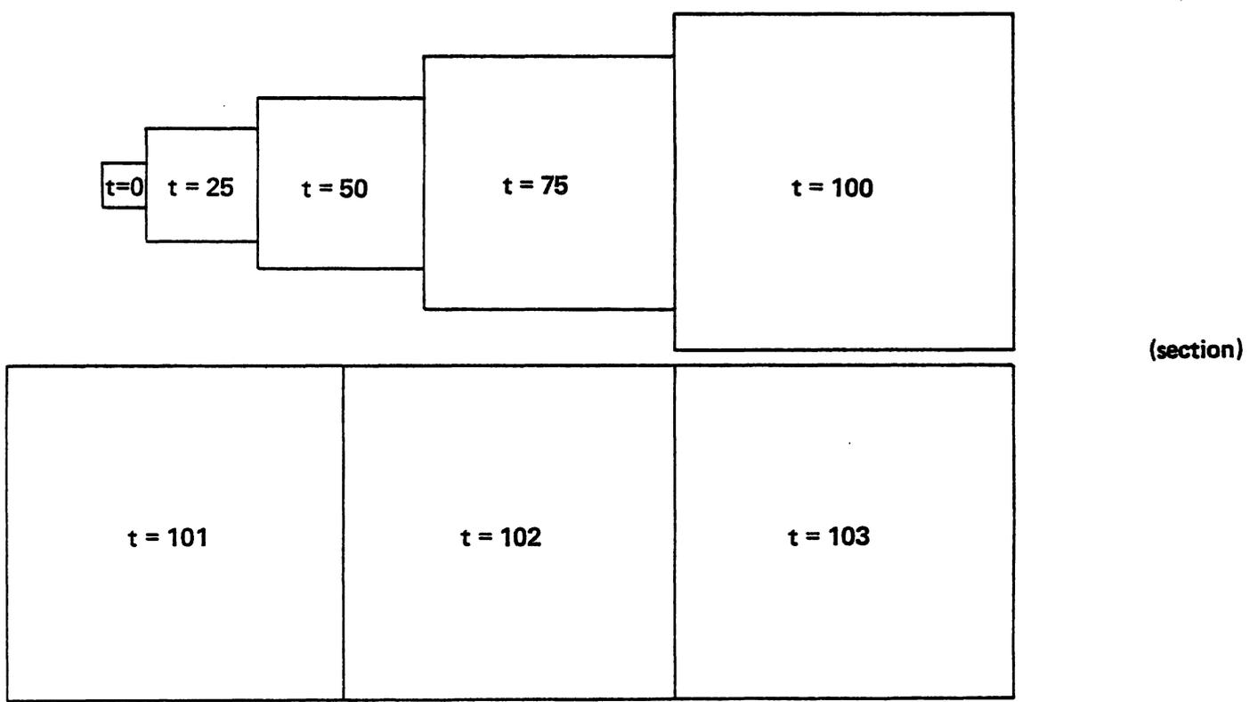
Figure 2.5: Examples of two-dimensional cellular automata that exhibit slow diffusive growth from small disordered regions. The cellular automaton rules shown are nine-neighbour square outer totalistic, with codes (a) 256746, (b) 736, (c) 291552.
