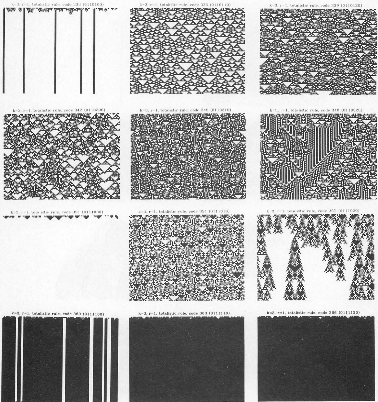
Fig. 4. Examples of the evolution of typical cellular automata with  $k = 3$  (three possible site values) and  $r = 1$  (only nearest neighbours included in time evolution rules). White squares represent value 0, grey squares value 1, and black squares value 2. The initial state is taken disordered, with each site having values 0, 1 and 2 with equal independent probabilities.
